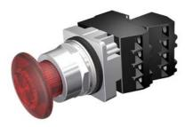
30mm Command/52, Chrome Finish Heavy Duty, Watertight/Oiltight Complete Metal Unit Illuminated Push-Pull Operator Full Voltage, 24V AC/DC Incandescent Lamp Mushroom Head Cap Small 1 3/4" (44.5 mm) Plastic, Red 3 Position Pull-Momentary/Push-Maintained 1 N.C.+1 N.C. Extra Late Break Heavy Duty Contacts, A600/P600 UL Listed, CSA Certified NEMA 1,3,3R,4,4X,12,13 & Automotive Standards
