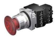
30mm Command/52, Chrome Finish Heavy Duty, Watertight/Oiltight Complete Metal Unit Illuminated Push-Pull Operator Full Voltage, 24V AC/DC LED Lamp Mushroom Head Cap Small 1 3/4" (44.5 mm) Plastic, Red 3 Position Pull-Momentary/Push-Maintained 1 N.C.+1 N.C. Extra Late Break Heavy Duty Contacts, A600/P600 UL Listed, CSA Certified NEMA 1,3,3R,4,4X,12,13 & Automotive Standards
