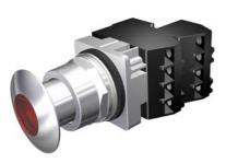
30mm Command/52, Chrome Finish Heavy Duty,Watertight/Oiltight Complete Metal Unit Illuminated Push-Pull Operator Full Voltage, 120V AC/DC Incandescent Lamp Mushroom Head Cap Small 1 3/4" (44.5 mm) Metal, Chrome with Red Lens 3 Position Momentary 1 N.C.+1 N.C. Extra Late Break Heavy Duty Contacts, A600/P600 UL Listed, CSA Certified NEMA 1,3,3R,4,4X,12,13 & Automotive Standards
