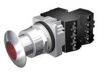
30mm Command/52, Chrome Finish Heavy Duty, Watertight/Oiltight Complete Metal Unit Illuminated Push-Pull Operator Full Voltage, 120V AC/DC LED Lamp Mushroom Head Cap Small 1 3/4" (44.5 mm) Metal, Chrome with Red Lens 3 Position Momentary 1 N.C.+1 N.C. Extra Late Break Heavy Duty Contacts, A600/P600 UL Listed, CSA Certified NEMA 1,3,3R,4,4X,12,13 & Automotive Standards
