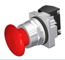
30mm Command/52, Chrome Finish Heavy Duty, Watertight/Oiltight Complete Metal Unit Push-Pull Operator Non-Illuminated Mushroom Head Cap Small 1 3/4" (44.5 mm) Plastic, Red 2 Position Maintained, Pull-to-Release with 1 N.C. Heavy Duty Contacts, A600/P600 UL Listed, CSA Certified NEMA 1,3,3R,4,4X,12,13 & Automotive Standards
