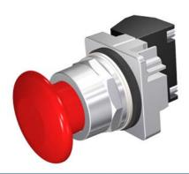
30mm Command/52, Chrome Finish Heavy Duty, Watertight/Oiltight Complete Metal Unit Push-Pull Operator Non-Illuminated Mushroom Head Cap Small 1 3/4" (44.5 mm) Plastic, Red 2 Position Maintained, Pull-to-Release with 1 N.O. - 1 N.C. Heavy Duty Contacts, A600/P600 UL Listed, CSA Certified NEMA 1,3,3R,4,4X,12,13 & Automotive Standards
