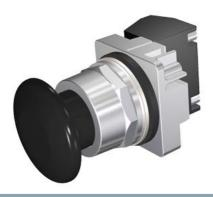
30mm Command/52, Chrome Finish Heavy Duty, Watertight/Oiltight Complete Metal Unit Push-Pull Operator Non-Illuminated Mushroom Head Cap Small 1 3/4" (44.5 mm) Plastic, Black 2 Position Maintained, Pull-to-Release with 1 N.O. - 1 N.C. Heavy Duty Contacts, A600/P600 UL Listed, CSA Certified NEMA 1,3,3R,4,4X,12,13 & Automotive Standards
