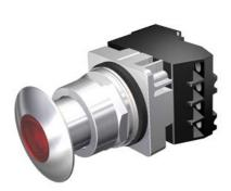
30mm Command/52, Chrome Finish Heavy Duty,Watertight/Oiltight Complete Metal Unit Illuminated Push-Pull Operator Full Voltage, 120V AC/DC LED Lamp Mushroom Head Cap Small 1 3/4" (44.5 mm) Metal, Chrome with Red Lens 2 Position Maintained, Pull-to-Release with 1 N.O. - 1 N.C. Heavy Duty Contacts, A600/P600 UL Listed, CSA Certified NEMA 1,3,3R,4,4X,12,13 & Automotive Standards
