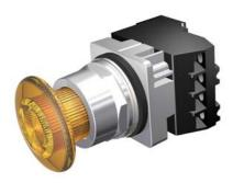
30mm Command/52, Chrome Finish Heavy Duty, Watertight/Oiltight Complete Metal Unit Illuminated Push-Pull Operator Full Voltage, 24V AC/DC LED Lamp Mushroom Head Cap Small 1 3/4" (44.5 mm) Plastic, Amber 2 Position Maintained, Pull-to-Release with 1 N.O. - 1 N.C. Heavy Duty Contacts, A600/P600 UL Listed, CSA Certified NEMA 1,3,3R,4,4X,12,13 & Automotive Standards
