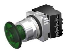
30mm Command/52, Chrome Finish Heavy Duty,Watertight/Oiltight Complete Metal Unit Illuminated Push-Pull Operator Full Voltage, 24V AC/DC LED Lamp Mushroom Head Cap Small 1 3/4" (44.5 mm) Plastic, Green 2 Position Maintained, Pull-to-Release with 1 N.O. - 1 N.C. Heavy Duty Contacts, A600/P600 UL Listed, CSA Certified NEMA 1,3,3R,4,4X,12,13 & Automotive Standards
