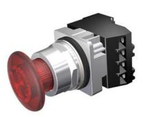
30mm Command/52, Chrome Finish Heavy Duty,Watertight/Oiltight Complete Metal Unit Illuminated Push-Pull Operator Full Voltage, 24V AC/DC LED Lamp Mushroom Head Cap Small 1 3/4" (44.5 mm) Plastic, Red 2 Position Maintained, Pull-to-Release with 1 N.O. - 1 N.C. Heavy Duty Contacts, A600/P600 UL Listed, CSA Certified NEMA 1,3,3R,4,4X,12,13 & Automotive Standards
