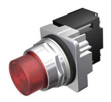
30mm Command/52, Chrome Finish Heavy Duty,Watertight/Oiltight Complete Metal Unit Illuminated Indicator Light Transformer type, 240V AC Incandescent Lamp, BA9s Plastic Lens, Red UL Listed, CSA Certified NEMA 1,3,3R,4,4X,12,13 & Automotive Standards
