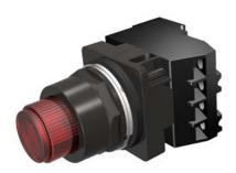
30mm BlackMax, Epoxy Coated Corrosion Resistant Complete Metal Unit PTT / Illuminated Pushbutton Transformer type, 600V AC Incandescent Lamp Extended Button Plastic Lens, Red 2 Position Momentary with 1 N.O. - 1 N.C. Heavy Duty Contacts, A600/P600 UL Listed, CSA Certified NEMA 1,3,3R,4,4X,12,13 & Automotive Standards
