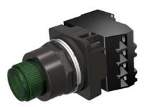
30mm BlackMax, Epoxy Coated Corrosion Resistant Complete Metal Unit PTT / Illuminated Pushbutton Full Voltage, 6V AC/DC Incandescent Lamp Extended Button Plastic Lens, Green 2 Position Momentary with 1 N.O. - 1 N.C. Heavy Duty Contacts, A600/P600 UL Listed, CSA Certified NEMA 1,3,3R,4,4X,12,13 & Automotive Standards
