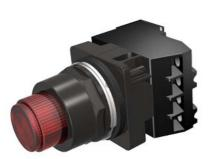
30mm BlackMax, Epoxy Coated Corrosion Resistant Complete Metal Unit PTT / Illuminated Pushbutton Full Voltage, 6V AC LED Lamp Extended Button Plastic Lens, Red 2 Position Momentary with 1 N.O. - 1 N.C. Heavy Duty Contacts, A600/P600 UL Listed, CSA Certified NEMA 1,3,3R,4,4X,12,13 & Automotive Standards
