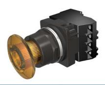
30mm BlackMax, Epoxy Coated Corrosion Resistant Complete Metal Unit Illuminated Twist-to-Release Transformer type, 240V AC Incandescent Lamp Mushroom Head Cap Small 1.79" (45 mm) Plastic Cap, Amber 2 Position Maintained, Twist-to-Release with 1 N.O. - 1 N.C. Heavy Duty Contacts, A600/P600 UL Listed, CSA Certified NEMA 1,3,3R,4,4X,12,13 & Automotive Standards
