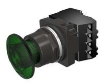
30mm BlackMax, Epoxy Coated Corrosion Resistant Complete Metal Unit Illuminated Twist-to-Release Transformer type, 240V AC Incandescent Lamp Mushroom Head Cap Small 1.79" (45 mm) Plastic Cap, Green 2 Position Maintained, Twist-to-Release with 1 N.O. - 1 N.C. Heavy Duty Contacts, A600/P600 UL Listed, CSA Certified NEMA 1,3,3R,4,4X,12,13 & Automotive Standards
