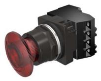
30mm BlackMax, Epoxy Coated Corrosion Resistant Complete Metal Unit Illuminated Twist-to-Release Transformer type, 240V AC Incandescent Lamp Mushroom Head Cap Small 1.79" (45 mm) Plastic Cap, Red 2 Position Maintained, Twist-to-Release with 1 N.O. - 1 N.C. Heavy Duty Contacts, A600/P600 UL Listed, CSA Certified NEMA 1,3,3R,4,4X,12,13 & Automotive Standards
