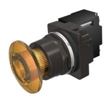
30mm BlackMax, Epoxy Coated Corrosion Resistant Metal Operator, Round Illuminated Twist-to-Release Transformer type, 120V AC LED Lamp Mushroom Head Cap Small 1.79" (45 mm) Plastic Cap, Amber 2 Position Maintained, Twist-to-Release UL Listed, CSA Certified NEMA 1,3,3R,4,4X,12,13 & Automotive Standards
