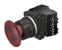
30mm BlackMax, Epoxy Coated Corrosion Resistant Complete Metal Unit Illuminated Twist-to-Release Full Voltage, 24V AC/DC LED Lamp Mushroom Head Cap Small 1.79" (45 mm) Plastic Cap, Red 2 Position Maintained, Twist-to-Release with 1 N.O. - 1 N.C. Heavy Duty Contacts, A600/P600 UL Listed, CSA Certified NEMA 1,3,3R,4,4X,12,13 & Automotive Standards
