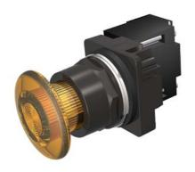
30mm BlackMax, Epoxy Coated Corrosion Resistant Complete Metal Unit Illuminated Push-Pull Operator Transformer type, 120V AC LED Lamp Mushroom Head Cap Small 1 3/4" (44.5 mm) Plastic, Amber 3 Position Pull-Momentary/Push-Maintained UL Listed, CSA Certified NEMA 1,3,3R,4,4X,12,13 & Automotive Standards
