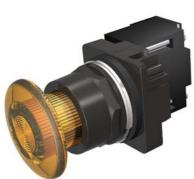
30mm BlackMax, Epoxy Coated Corrosion Resistant Complete Metal Unit Illuminated Push-Pull Operator Full Voltage, 24V AC/DC LED Lamp Mushroom Head Cap Small 1 3/4" (44.5 mm) Plastic, Amber 3 Position Pull-Momentary/Push-Maintained UL Listed, CSA Certified NEMA 1,3,3R,4,4X,12,13 & Automotive Standards
