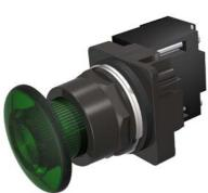
30mm BlackMax, Epoxy Coated Corrosion Resistant Complete Metal Unit Illuminated Push-Pull Operator Full Voltage, 24V AC/DC Incandescent Lamp Mushroom Head Cap Small 1 3/4" (44.5 mm) Plastic, Green 3 Position Pull-Momentary/Push-Maintained UL Listed, CSA Certified NEMA 1,3,3R,4,4X,12,13 & Automotive Standards
