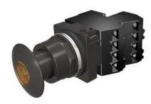
30mm BlackMax, Epoxy Coated Corrosion Resistant Complete Metal Unit Illuminated Push-Pull Operator Full Voltage, 6V AC LED Lamp Mushroom Head Cap Small 1 3/4" (44.5 mm) Metal, Black with Amber Lens 3 Position Pull-Momentary/Push-Maintained 1 N.C.+1 N.C. Extra Late Break Heavy Duty Contacts, A600/P600 UL Listed, CSA Certified NEMA 1,3,3R,4,4X,12,13 & Automotive Standards
