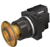
30mm BlackMax, Epoxy Coated Corrosion Resistant Complete Metal Unit Illuminated Push-Pull Operator Full Voltage, 24V AC/DC Incandescent Lamp Mushroom Head Cap Small 1 3/4" (44.5 mm) Plastic, Amber 3 Position Momentary UL Listed, CSA Certified NEMA 1,3,3R,4,4X,12,13 & Automotive Standards
