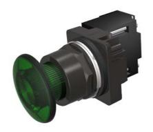
30mm BlackMax, Epoxy Coated Corrosion Resistant Complete Metal Unit Illuminated Push-Pull Operator Full Voltage, 24V AC/DC LED Lamp Mushroom Head Cap Small 1 3/4" (44.5 mm) Plastic, Green 3 Position Momentary UL Listed, CSA Certified NEMA 1,3,3R,4,4X,12,13 & Automotive Standards
