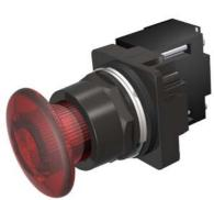
30mm BlackMax, Epoxy Coated Corrosion Resistant Complete Metal Unit Illuminated Push-Pull Operator Full Voltage, 24V AC/DC LED Lamp Mushroom Head Cap Small 1 3/4" (44.5 mm) Plastic, Red 3 Position Momentary UL Listed, CSA Certified NEMA 1,3,3R,4,4X,12,13 & Automotive Standards
