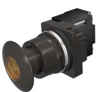
30mm BlackMax, Epoxy Coated Corrosion Resistant Complete Metal Unit Illuminated Push-Pull Operator Full Voltage, 12V AC/DC Incandescent Lamp Mushroom Head Cap Small 1 3/4" (44.5 mm) Metal, Black with Amber Lens 3 Position Momentary UL Listed, CSA Certified NEMA 1,3,3R,4,4X,12,13 & Automotive Standards
