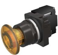
30mm BlackMax, Epoxy Coated Corrosion Resistant Complete Metal Unit Illuminated Push-Pull Operator Full Voltage, 6V AC LED Lamp Mushroom Head Cap Small 1 3/4" (44.5 mm) Plastic, Amber 3 Position Momentary UL Listed, CSA Certified NEMA 1,3,3R,4,4X,12,13 & Automotive Standards
