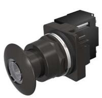
30mm BlackMax, Epoxy Coated Corrosion Resistant Complete Metal Unit Illuminated Push-Pull Operator Transformer type, 600V AC LED Lamp Mushroom Head Cap Small 1 3/4" (44.5 mm) Metal, Black with Clear Lens 2 Position Maintained, Pull-to-Release UL Listed, CSA Certified NEMA 1,3,3R,4,4X,12,13 & Automotive Standards
