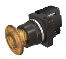
30mm BlackMax, Epoxy Coated Corrosion Resistant Complete Metal Unit Illuminated Push-Pull Operator Transformer type, 240V AC LED Lamp Mushroom Head Cap Small 1 3/4" (44.5 mm) Plastic, Amber 2 Position Maintained, Pull-to-Release UL Listed, CSA Certified NEMA 1,3,3R,4,4X,12,13 & Automotive Standards
