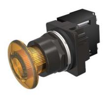
30mm BlackMax, Epoxy Coated Corrosion Resistant Complete Metal Unit Illuminated Push-Pull Operator Full Voltage, 120V AC/DC LED Lamp Mushroom Head Cap Small 1 3/4" (44.5 mm) Plastic, Amber 2 Position Maintained, Pull-to-Release UL Listed, CSA Certified NEMA 1,3,3R,4,4X,12,13 & Automotive Standards
