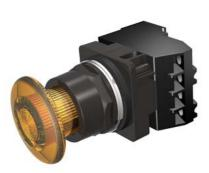
30mm BlackMax, Epoxy Coated Corrosion Resistant Complete Metal Unit Illuminated Push-Pull Operator Full Voltage, 24V AC/DC LED Lamp Mushroom Head Cap Small 1 3/4" (44.5 mm) Plastic, Amber 2 Position Maintained, Pull-to-Release with 1 N.O. - 1 N.C. Heavy Duty Contacts, A600/P600 UL Listed, CSA Certified NEMA 1,3,3R,4,4X,12,13 & Automotive Standards
