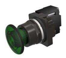
30mm BlackMax, Epoxy Coated Corrosion Resistant Complete Metal Unit Illuminated Push-Pull Operator Full Voltage, 24V AC/DC Incandescent Lamp Mushroom Head Cap Small 1 3/4" (44.5 mm) Plastic, Green 2 Position Maintained, Pull-to-Release UL Listed, CSA Certified NEMA 1,3,3R,4,4X,12,13 & Automotive Standards
