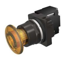
30mm BlackMax, Epoxy Coated Corrosion Resistant Complete Metal Unit Illuminated Push-Pull Operator Full Voltage, 12V AC/DC Incandescent Lamp Mushroom Head Cap Small 1 3/4" (44.5 mm) Plastic, Amber 2 Position Maintained, Pull-to-Release UL Listed, CSA Certified NEMA 1,3,3R,4,4X,12,13 & Automotive Standards
