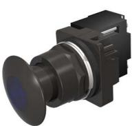
30mm BlackMax, Epoxy Coated Corrosion Resistant Complete Metal Unit Illuminated Push-Pull Operator Full Voltage, 12V AC/DC Incandescent Lamp Mushroom Head Cap Small 1 3/4" (44.5 mm) Metal, Black with Blue Lens 2 Position Maintained, Pull-to-Release UL Listed, CSA Certified NEMA 1,3,3R,4,4X,12,13 & Automotive Standards
