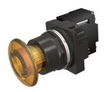
30mm BlackMax, Epoxy Coated Corrosion Resistant Complete Metal Unit Illuminated Push-Pull Operator Full Voltage, 6V AC LED Lamp Mushroom Head Cap Small 1 3/4" (44.5 mm) Plastic, Amber 2 Position Maintained, Pull-to-Release UL Listed, CSA Certified NEMA 1,3,3R,4,4X,12,13 & Automotive Standards
