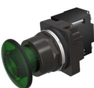
30mm BlackMax, Epoxy Coated Corrosion Resistant Complete Metal Unit Illuminated Push-Pull Operator Full Voltage, 6V AC LED Lamp Mushroom Head Cap Small 1 3/4" (44.5 mm) Plastic, Green 2 Position Maintained, Pull-to-Release UL Listed, CSA Certified NEMA 1,3,3R,4,4X,12,13 & Automotive Standards
