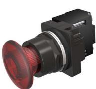
30mm BlackMax, Epoxy Coated Corrosion Resistant Complete Metal Unit Illuminated Push-Pull Operator Full Voltage, 6V AC LED Lamp Mushroom Head Cap Small 1 3/4" (44.5 mm) Plastic, Red 2 Position Maintained, Pull-to-Release UL Listed, CSA Certified NEMA 1,3,3R,4,4X,12,13 & Automotive Standards
