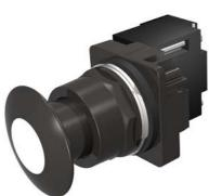
30mm BlackMax, Epoxy Coated Corrosion Resistant Complete Metal Unit Illuminated Push-Pull Operator Full Voltage, 6V AC/DC Incandescent Lamp Mushroom Head Cap Small 1 3/4" (44.5 mm) Metal, Black with White Lens 2 Position Maintained, Pull-to-Release UL Listed, CSA Certified NEMA 1,3,3R,4,4X,12,13 & Automotive Standards
