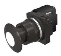
30mm BlackMax, Epoxy Coated Corrosion Resistant Complete Metal Unit Illuminated Push-Pull Operator Full Voltage, 6V AC LED Lamp Mushroom Head Cap Small 1 3/4" (44.5 mm) Metal, Black with White Lens 2 Position Maintained, Pull-to-Release UL Listed, CSA Certified NEMA 1,3,3R,4,4X,12,13 & Automotive Standards
