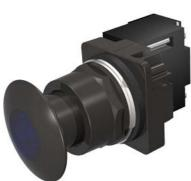
30mm BlackMax, Epoxy Coated Corrosion Resistant Complete Metal Unit Illuminated Push-Pull Operator Full Voltage, 6V AC/DC Incandescent Lamp Mushroom Head Cap Small 1 3/4" (44.5 mm) Metal, Black with Blue Lens 2 Position Maintained, Pull-to-Release UL Listed, CSA Certified NEMA 1,3,3R,4,4X,12,13 & Automotive Standards
