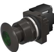
30mm BlackMax, Epoxy Coated Corrosion Resistant Complete Metal Unit Illuminated Push-Pull Operator Full Voltage, 6V AC/DC Incandescent Lamp Mushroom Head Cap Small 1 3/4" (44.5 mm) Metal, Black with Green Lens 2 Position Maintained, Pull-to-Release UL Listed, CSA Certified NEMA 1,3,3R,4,4X,12,13 & Automotive Standards
