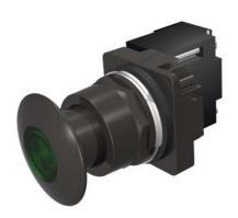
30mm BlackMax, Epoxy Coated Corrosion Resistant Complete Metal Unit Illuminated Push-Pull Operator Full Voltage, 6V AC LED Lamp Mushroom Head Cap Small 1 3/4" (44.5 mm) Metal, Black with Green Lens 2 Position Maintained, Pull-to-Release UL Listed, CSA Certified NEMA 1,3,3R,4,4X,12,13 & Automotive Standards
