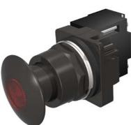
30mm BlackMax, Epoxy Coated Corrosion Resistant Complete Metal Unit Illuminated Push-Pull Operator Full Voltage, 6V AC/DC Incandescent Lamp Mushroom Head Cap Small 1 3/4" (44.5 mm) Metal, Black with Red Lens 2 Position Maintained, Pull-to-Release UL Listed, CSA Certified NEMA 1,3,3R,4,4X,12,13 & Automotive Standards
