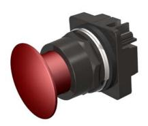
30mm BlackMax, Epoxy Coated Corrosion Resistant Metal Operator, Round Push-Pull Operator Non-Illuminated Mushroom Head Cap Small 1.73" (44 mm) Metal, Anodized Red 2 Position Maintained, Pull-to-Release UL Listed, CSA Certified NEMA 1,3,3R,4,4X,12,13 & Automotive Standards
