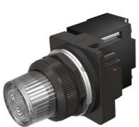
30mm BlackMax, Epoxy Coated Corrosion Resistant Complete Metal Unit Illuminated Indicator Light Transformer type, 600V AC Incandescent Lamp, BA9s Glass Lens, Clear UL Listed, CSA Certified NEMA 1,3,3R,4,4X,12,13 & Automotive Standards
