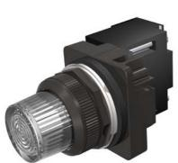
30mm BlackMax, Epoxy Coated Corrosion Resistant Complete Metal Unit Illuminated Indicator Light Transformer type, 600V AC LED Lamp, BA9s Glass Lens, Clear UL Listed, CSA Certified NEMA 1,3,3R,4,4X,12,13 & Automotive Standards
