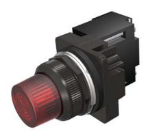
30mm BlackMax, Epoxy Coated Corrosion Resistant Complete Metal Unit Illuminated Indicator Light Transformer type, 600V AC Super Bright LED Lamp, BA9s Glass Lens, Red UL Listed, CSA Certified NEMA 1,3,3R,4,4X,12,13 & Automotive Standards
