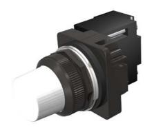
30mm BlackMax, Epoxy Coated Corrosion Resistant Complete Metal Unit Illuminated Indicator Light Transformer type, 480V AC Incandescent Lamp, BA9s Glass Lens, White UL Listed, CSA Certified NEMA 1,3,3R,4,4X,12,13 & Automotive Standards
